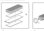
$\bigcirc$  Install thermal silicon M 2 SSD • Put the aluminum alloy radiator ∠) on two Rubber Rim and heatsink
