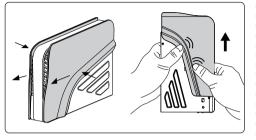
Press the white cover and slide it forward to remove both white covers from the chassis
